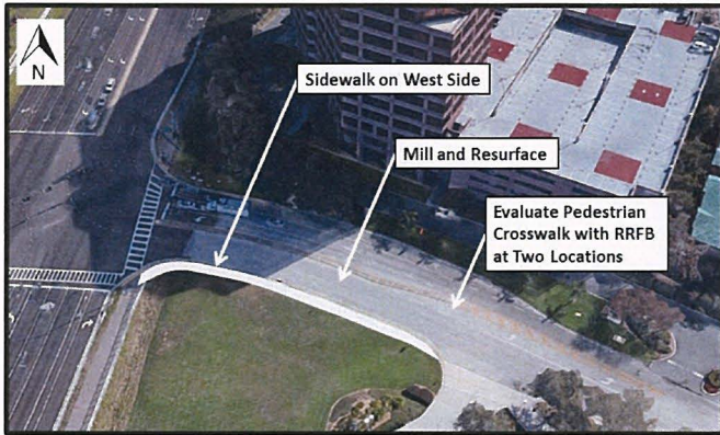
Mill and Resurfacing Sidewalks and Mid-block Crossings with RRFBs
